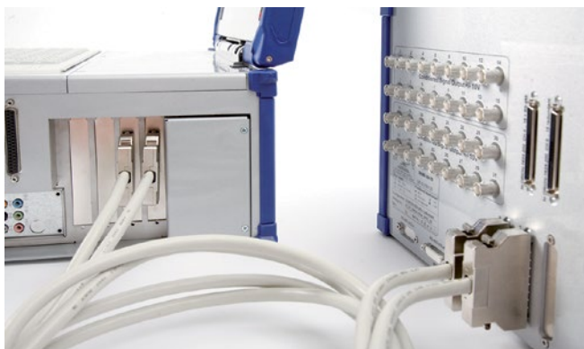
Extra 32 channel signal conditioning to expand a 16 channel instrument to a total of 48 channels
