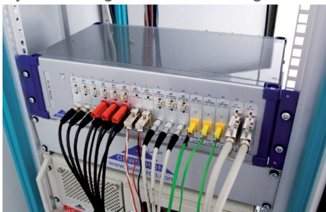
Signal connection to HSI/DAQP modules
