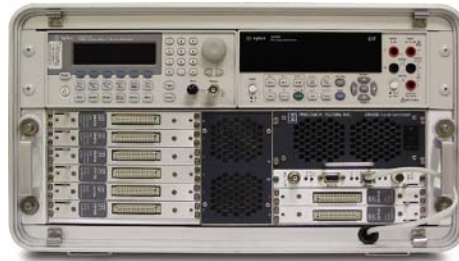
Test Subsystem with 28008-M3 installed in optional transit case.
