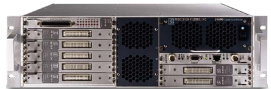
28008-M3 compact 8-slot chassis requires only 5.25 inches of rack space.
