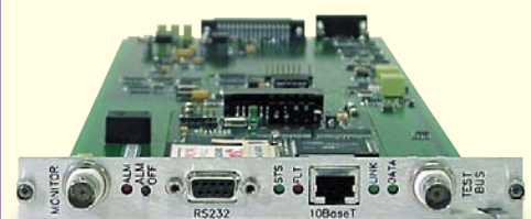
Backplane Interface Card (BIF) is installed in a dedicated card slot in the 28000 mainframe.
