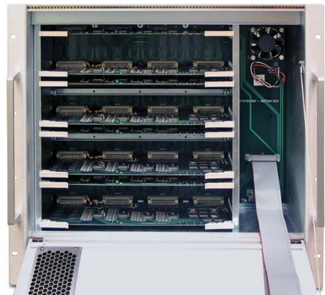
Figure 10 464kB Interstage Cards Installed
